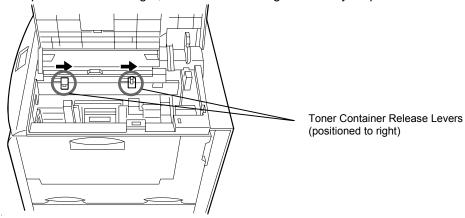
**4.** Align the ends of the toner container with the grooves to the left and right inside the printer as shown in the figure and install.
